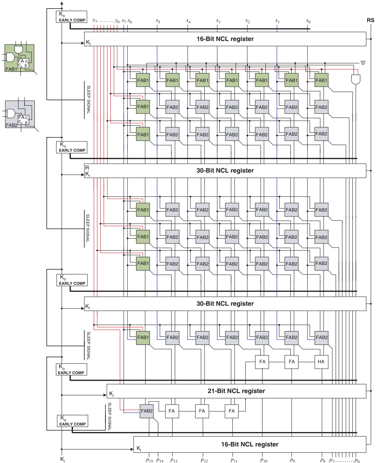
Fig. 11. 8 × 8 MTCMOS NCL array multiplier.
