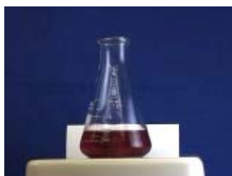
Figure 6. Photograph of a colloidal suspension of Au nanoparticles in water.
